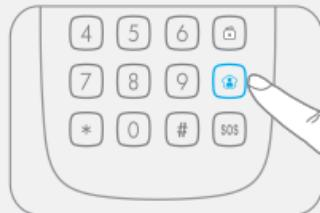
When the alarm panel receives the signal, the siren beeps once and the Home Mode indicator lights up: the alarm system is now in Home Mode.
