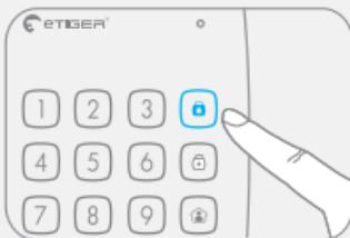
When the alarm panel receives the signal, the siren beeps once and the Arm indicator on the control panel lights up. The alarm system is now armed.
