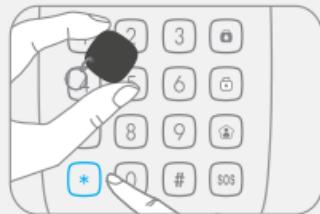
The RFID reader turns off when a RFID tag is swiped in front of it, when the key [\*] is pressed again on the keypad, or after 10 seconds without operation.
